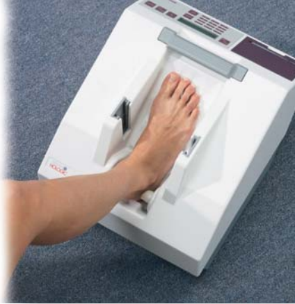
View of patient's heel positioned properly between transducers. Direct contact with heel produces an accurate measurement of heel width, not an estimation like water-based systems.
