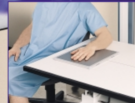
A wide range of cross-table procedures can be performed by rotating the tubestand on the vertical axis and utilizing the tube trunnion rings.
